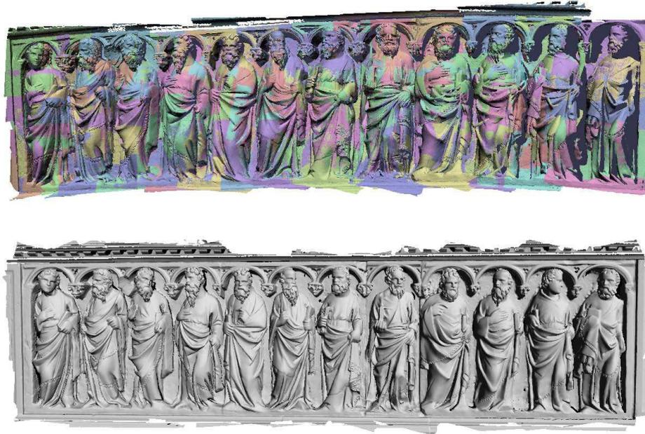
Figure 5. The coarse alignment obtained over a set of range maps representing a bas-relief (top) and the final model (bottom) obtained after automatic completion of all overlapping-pairs
