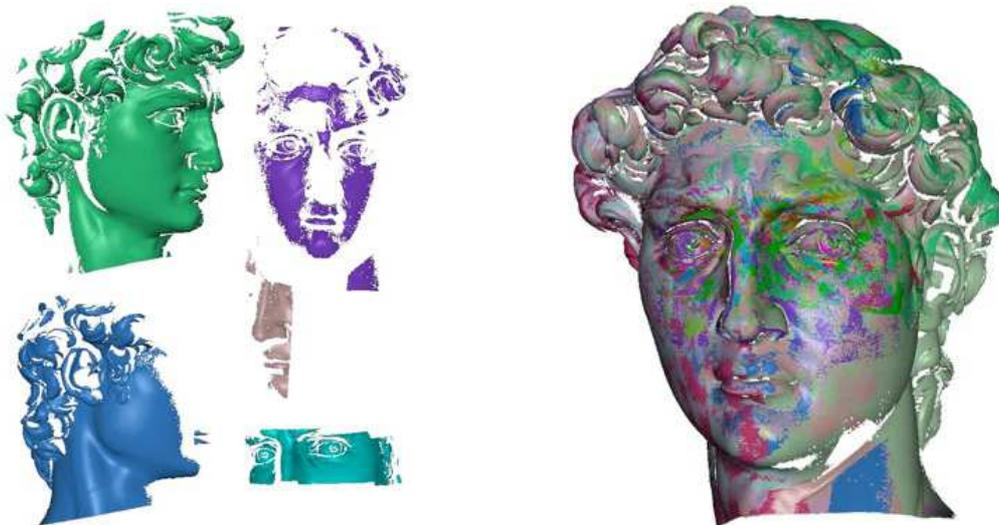
Figure 4. The alignment step brings non-referenced range-maps (left) and put them together in a single common reference frame (right).
