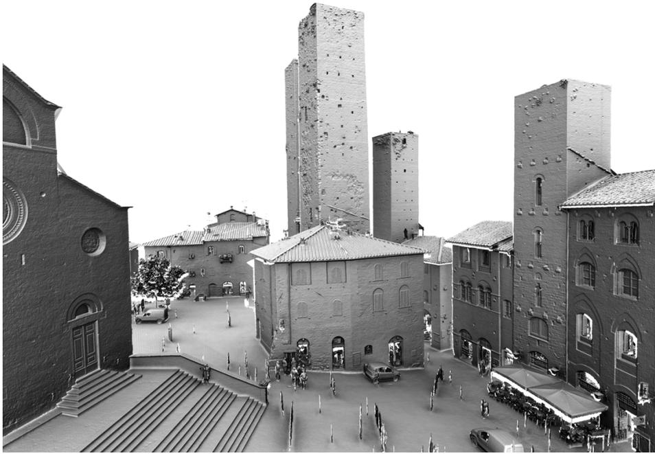
Figure 6. Domesquare at S. Gimignano (Italy) acquired using a terrestrial time of flight laser scanner. Cleaned-up model after alignment, cleaning and merging. Rendering using directional lighting and ambient occlusion. Image courtesy of ISTI-CNR.
