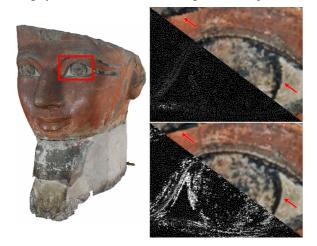
**Figure 9:** *Adaptive point cloud refinement. Left: complete model. Middle: image blending on original point cloud. Right: image blending on adaptively refined point cloud.*
