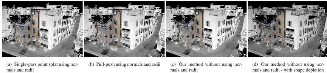
Figure 10: Sirmione (100Mpts): (a) single-pass point splat and (b) pull-push infilling algorithm using normals and radii, our method without using normals and radii, without (c) and with (d) our shape depiction shading approach.
